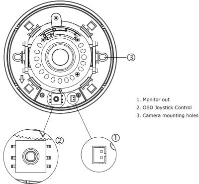
Figure 2-3 Camera adjustment controls
